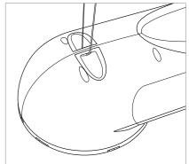
Figure 4. Attaching a safety wire.
